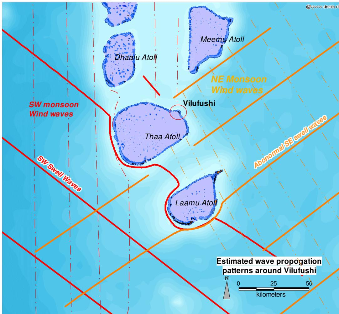
**Figure 2.1 Estimated (predominant) wave propagation patterns around Vilufushi: the island enjoys protection from southern swell waves due to its location, atoll shape and line-up of atolls.**
